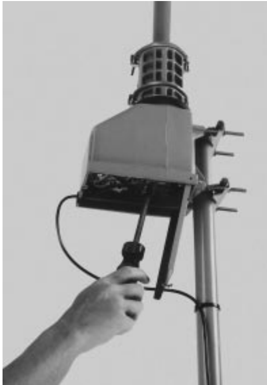
Fig. 8-1. The mast-mounted drive unit of an antenna rotor.
