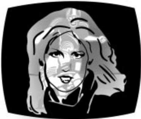
Fig. 11-4. The most common symptom of adjacent channel interference.
