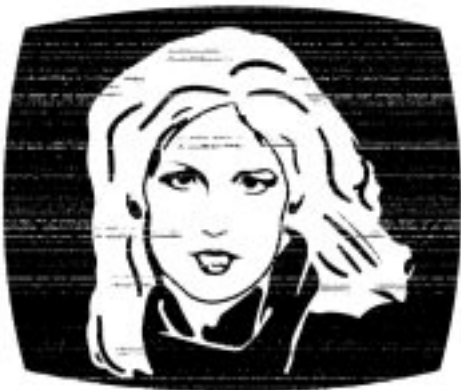
Fig. 11-8. Bright static caused by electromagnetic interference.
