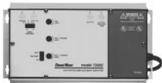
Fig. 10-4b. When many outlets (more than 4) are required, a distribution amplifier should be used.
