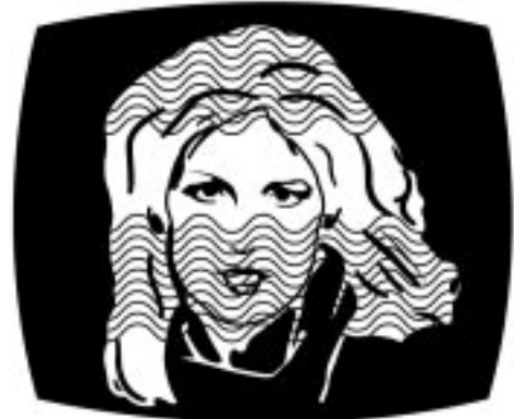
Fig. 11-9. A herringbone pattern caused by FM interference.
