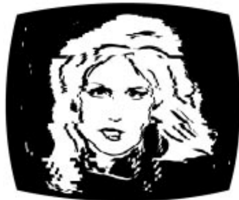
Fig. 11-3. Blurred and smearred TV pictures.
